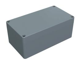
Hammond enclosure, NEMA 4/4X, 220 x 120 x 91mm (HxWxD), fiberglass reinforced polyester, RAL 7000 light gray, screw cover, purchase subpanel separately.
