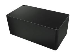
Hammond enclosure, NEMA 4/4X, 220 x 120 x 91mm (HxWxD), fiberglass reinforced polyester, black, screw cover, purchase subpanel separately.
