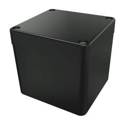
Hammond enclosure, NEMA 4/4X,  $81 \times 76 \times 75 \text{mm}$  (HxWxD), fiberglass reinforced polyester, black, screw cover, purchase subpanel separately.
