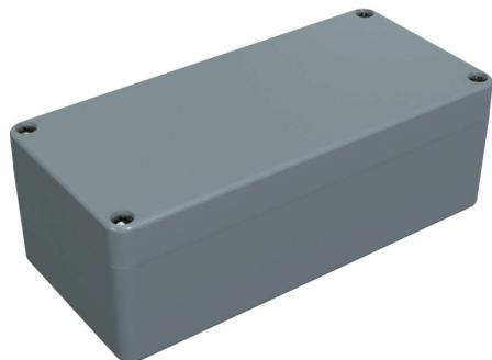
Hammond enclosure, NEMA 4/4X, 160 x 75 x 55mm (HxWxD), fiberglass reinforced polyester, RAL 7000 light gray, screw cover, purchase subpanel separately.
