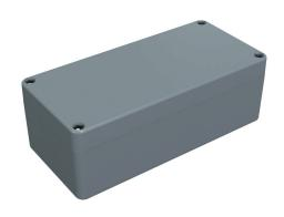
Hammond enclosure, NEMA 4/4X,  $160 \times 75 \times 55$ mm (HxWxD), fiberglass reinforced polyester, RAL 7000 light gray, screw cover, purchase subpanel separately.
