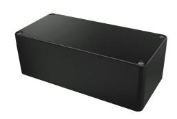
Hammond enclosure, NEMA 4/4X,  $160 \times 75 \times 55$ mm (HxWxD), fiberglass reinforced polyester, black, screw cover, purchase subpanel separately.
