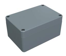
Hammond enclosure, NEMA 4/4X,  $110 \times 75 \times 55$ mm (HxWxD), fiberglass reinforced polyester, RAL 7000 light gray, screw cover, purchase subpanel separately.
