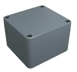
Hammond enclosure, NEMA 4/4X, 80 x 75 x 55mm (HxWxD), fiberglass reinforced polyester, RAL 7000 light gray, screw cover, purchase subpanel separately.
