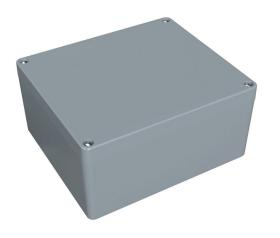
Hammond enclosure, NEMA 4/4X/6/6P, 230 x 200 x 110mm (HxWxD), die-cast aluminum alloy, RAL 7001 light gray, powder coat finish, screw cover, purchase subpanel separately.
