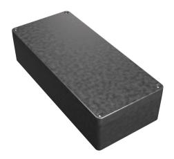
Hammond enclosure, NEMA 4/4X/6/6P, 360 x 160 x 90mm (HxWxD), die-cast aluminum alloy, screw cover, purchase subpanel separately.
