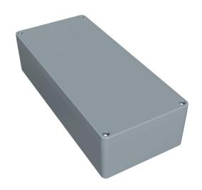
Hammond enclosure, NEMA 4/4X/6/6P, 360 x 160 x 90mm (HxWxD), die-cast aluminum alloy, RAL 7001 light gray, powder coat finish, screw cover, purchase subpanel separately.
