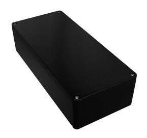
Hammond enclosure, NEMA 4/4X/6/6P, 360 x 160 x 90mm (HxWxD), die-cast aluminum alloy, black, powder coat finish, screw cover, purchase subpanel separately.
