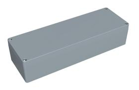
Hammond enclosure, NEMA 4/4X/6/6P, 360 x 122 x 80mm (HxWxD), die-cast aluminum alloy, RAL 7001 light gray, powder coat finish, screw cover, purchase subpanel separately.
