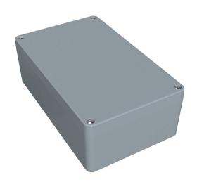
Hammond enclosure, NEMA 4/4X/6/6P, 260 x 160 x 90mm (HxWxD), die-cast aluminum alloy, RAL 7001 light gray, powder coat finish, screw cover, purchase subpanel separately.
