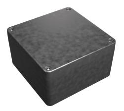
Hammond enclosure, NEMA 4/4X/6/6P, 160 x 160 x 90mm (HxWxD), die-cast aluminum alloy, screw cover, purchase subpanel separately.
