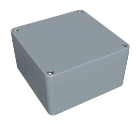
Hammond enclosure, NEMA 4/4X/6/6P, 160 x 160 x 90mm (HxWxD), die-cast aluminum alloy, RAL 7001 light gray, powder coat finish, screw cover, purchase subpanel separately.
