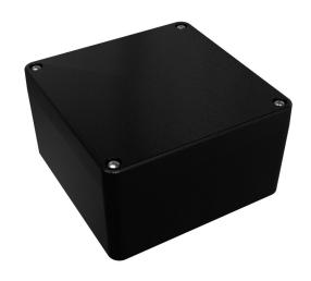
Hammond enclosure, NEMA 4/4X/6/6P, 160 x 160 x 90mm (HxWxD), die-cast aluminum alloy, black, powder coat finish, screw cover, purchase subpanel separately.
