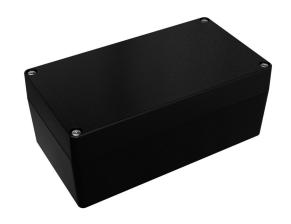
Hammond enclosure, NEMA 4/4X/6/6P, 221 x 121 x 90mm (HxWxD), die-cast aluminum alloy, black, powder coat finish, screw cover, purchase subpanel separately.
