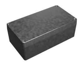
Hammond enclosure, NEMA 4/4X/6/6P, 221 x 121 x 81mm (HxWxD), die-cast aluminum alloy, screw cover, purchase subpanel separately.
