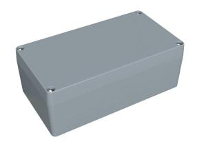
Hammond enclosure, NEMA 4/4X/6/6P, 221 x 121 x 81mm (HxWxD), die-cast aluminum alloy, RAL 7001 light gray, powder coat finish, screw cover, purchase subpanel separately.
