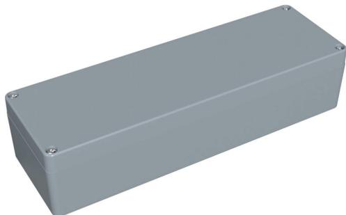
Hammond enclosure, NEMA 4/4X/6/6P, 250 x 80 x 57mm (HxWxD), die-cast aluminum alloy, RAL 7001 light gray, powder coat finish, screw cover, purchase subpanel separately.
