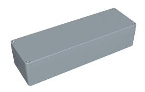
Hammond enclosure, NEMA 4/4X/6/6P, 250 x 80 x 57mm (HxWxD), die-cast aluminum alloy, RAL 7001 light gray, powder coat finish, screw cover, purchase subpanel separately.
