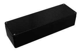
Hammond enclosure, NEMA 4/4X/6/6P, 250 x 80 x 57mm (HxWxD), die-cast aluminum alloy, black, powder coat finish, screw cover, purchase subpanel separately.
