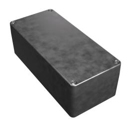
Hammond enclosure, NEMA 4/4X/6/6P, 175 x 80 x 60mm (HxWxD), die-cast aluminum alloy, screw cover.
