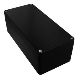
Hammond enclosure, NEMA 4/4X/6/6P, 175 x 80 x 60mm (HxWxD), die-cast aluminum alloy, black, powder coat finish, screw cover.
