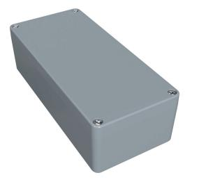
Hammond enclosure, NEMA 4/4X/6/6P, 175 x 80 x 52mm (HxWxD), die-cast aluminum alloy, RAL 7001 light gray, powder coat finish, screw cover.
