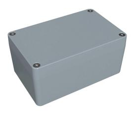
Hammond enclosure, NEMA 4/4X/6/6P, 125 x 80 x 59mm (HxWxD), die-cast aluminum alloy, RAL 7001 light gray, powder coat finish, screw cover, purchase subpanel separately.
