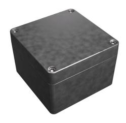
Hammond enclosure, NEMA 4/4X/6/6P, 122 x 120 x 82mm (HxWxD), die-cast aluminum alloy, screw cover, purchase subpanel separately.
