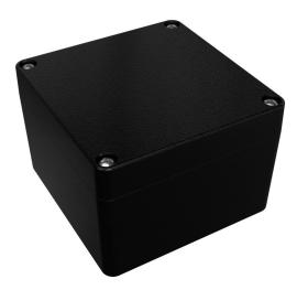
Hammond enclosure, NEMA 4/4X/6/6P, 122 x 120 x 82mm (HxWxD), die-cast aluminum alloy, black, powder coat finish, screw cover, purchase subpanel separately.
