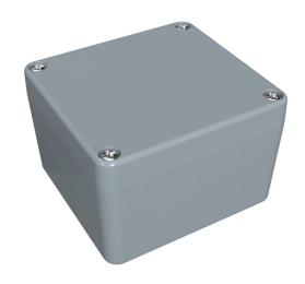
Hammond enclosure, NEMA 4/4X/6/6P, 80 x 75 x 52mm (HxWxD), die-cast aluminum alloy, RAL 7001 light gray, powder coat finish, screw cover.
