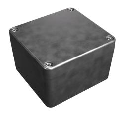
Hammond enclosure, NEMA 4/4X/6/6P, 80 x 75 x 52mm (HxWxD), die-cast aluminum alloy, screw cover, purchase subpanel separately.
