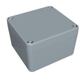
Hammond enclosure, NEMA 4/4X/6/6P,  $80 \times 75 \times 52$ mm (HxWxD), die-cast aluminum alloy, RAL 7001 light gray, powder coat finish, screw cover, purchase subpanel separately.
