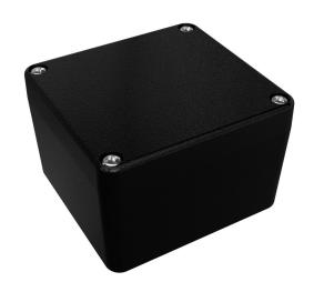
Hammond enclosure, NEMA 4/4X/6/6P, 80 x 75 x 52mm (HxWxD), die-cast aluminum alloy, black, powder coat finish, screw cover, purchase subpanel separately.
