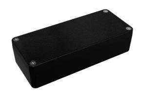
Hammond enclosure, NEMA 4/4X/6/6P, 150 x 64 x 36mm (HxWxD), die-cast aluminum alloy, black, powder coat finish, screw cover.
