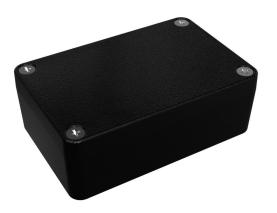
Hammond enclosure, NEMA 4/4X/6/6P, 98 x 64 x 34mm (HxWxD), die-cast aluminum alloy, black, powder coat finish, screw cover.
