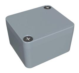
Hammond enclosure, NEMA 4/4X/6/6P, 50 x 45 x 30mm (HxWxD), die-cast aluminum alloy, RAL 7001 light gray, powder coat finish, screw cover.
