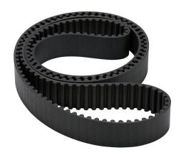
SureMotion timing belt, 8mm 8M pitch, 30mm wide, 198 tooth, 1584mm pitch length (circumference), neoprene, fiberglass reinforced.
