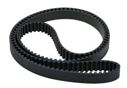
SureMotion timing belt, 8mm 8M pitch, 20mm wide, 198 tooth, 1584mm pitch length (circumference), neoprene, fiberglass reinforced.
