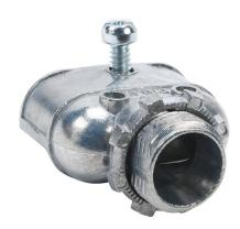
Halex fitting, zinc die cast, straight duplex, 3/8in trade size, screw clamp conduit connection. Package of 25. For use with flexible metal conduit (FMC), AC cable (BX), MC cable, (NM-B) cable. Screws and locknut included.
