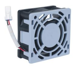
WEG Electric CFW500 series main cooling fan, replacement,  $60 \times 60 \times 25$ mm, 12 VDC. For use with WEG CFW500 series IP66 230 VAC 7-1/2hp and below, 460 VAC 10hp and below AC drives.
