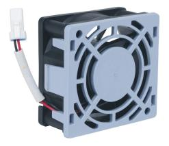
WEG Electric CFW500 series main cooling fan, replacement, 60 x 60 x 25mm, 12 VDC. For use with WEG CFW500 series IP66 230 VAC 7-1/2hp and below, 460 VAC 10hp and below AC drives.
