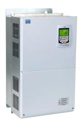
WEG Electric CFW500 series AC high-performance drive, enclosed, 460 VAC, 60hp with 3-phase input, SVC, V/Hz, VVW, FOC, encoder or torque mode, F frame, RS-485, integrated dynamic braking. Optional communication and STO modules available.
