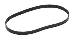
SureMotion timing belt, 0.08in MXL pitch, 1/4in wide, 156 tooth, 12.5in pitch length (circumference), polyurethane, polyester reinforced. Package of 3.
