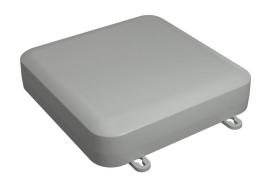
Hammond enclosure, NEMA 4/4X/6/6P/12/13, 200 x 200 x 45mm (HxWxD), polycarbonate, RAL 7035 light gray, screw cover.
