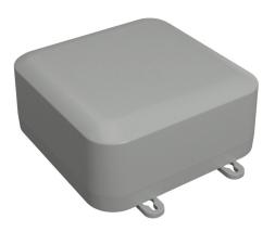
Hammond enclosure, NEMA 4/4X/6/6P/12/13, 160 x 160 x 70mm (HxWxD), polycarbonate, RAL 7035 light gray, screw cover.
