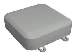
Hammond enclosure, NEMA 4/4X/6/6P/12/13, 160 x 160 x 45mm (HxWxD), polycarbonate, RAL 7035 light gray, screw cover.
