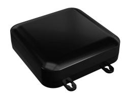
Hammond enclosure, NEMA 4/4X/6/6P/12/13,  $160 \times 160 \times 45$ mm (HxWxD), polycarbonate, black, screw cover.
