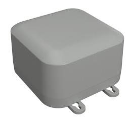
Hammond enclosure, NEMA 4/4X/6/6P/12/13,  $120 \times 120 \times 70$ mm (HxWxD), polycarbonate, RAL 7035 light gray, screw cover.
