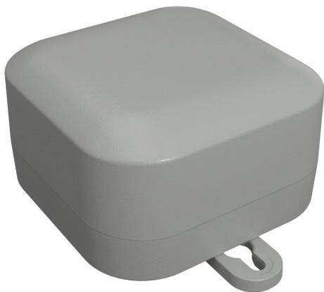
Hammond enclosure, NEMA 4/4X/6/6P/12/13, 80 x 80 x 45mm (HxWxD), polycarbonate, RAL 7035 light gray, screw cover.
