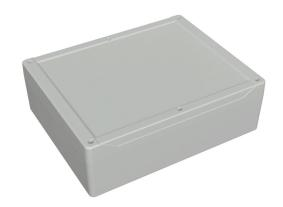
Hammond enclosure, NEMA 4/4X/6/6P/12/13, 299 x 240 x 95mm (HxWxD), ABS plastic, RAL 7035 light gray, screw cover with smooth recess, purchase subpanel separately.
