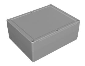
Hammond enclosure, NEMA 4/4X/6/6P/12/13, 299 x 240 x 120mm (HxWxD), polycarbonate, RAL 7035 light gray, screw cover with smooth recess, purchase subpanel separately.
