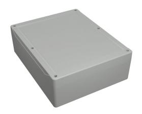
Hammond enclosure, NEMA 4/4X/6/6P/12/13, 299 x 240 x 95mm (HxWxD), polycarbonate, RAL 7035 light gray, screw cover with smooth recess, purchase subpanel separately.
