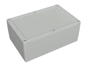
Hammond enclosure, NEMA 4/4X/6/6P/12/13, 299 x 200 x 120mm (HxWxD), ABS plastic, RAL 7035 light gray, screw cover with smooth recess, purchase subpanel separately.
